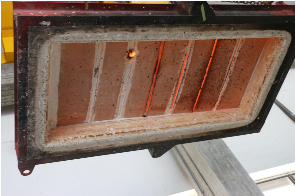
Photo 7: The Exposed Face of the Test Assembly Immediately After Testing
