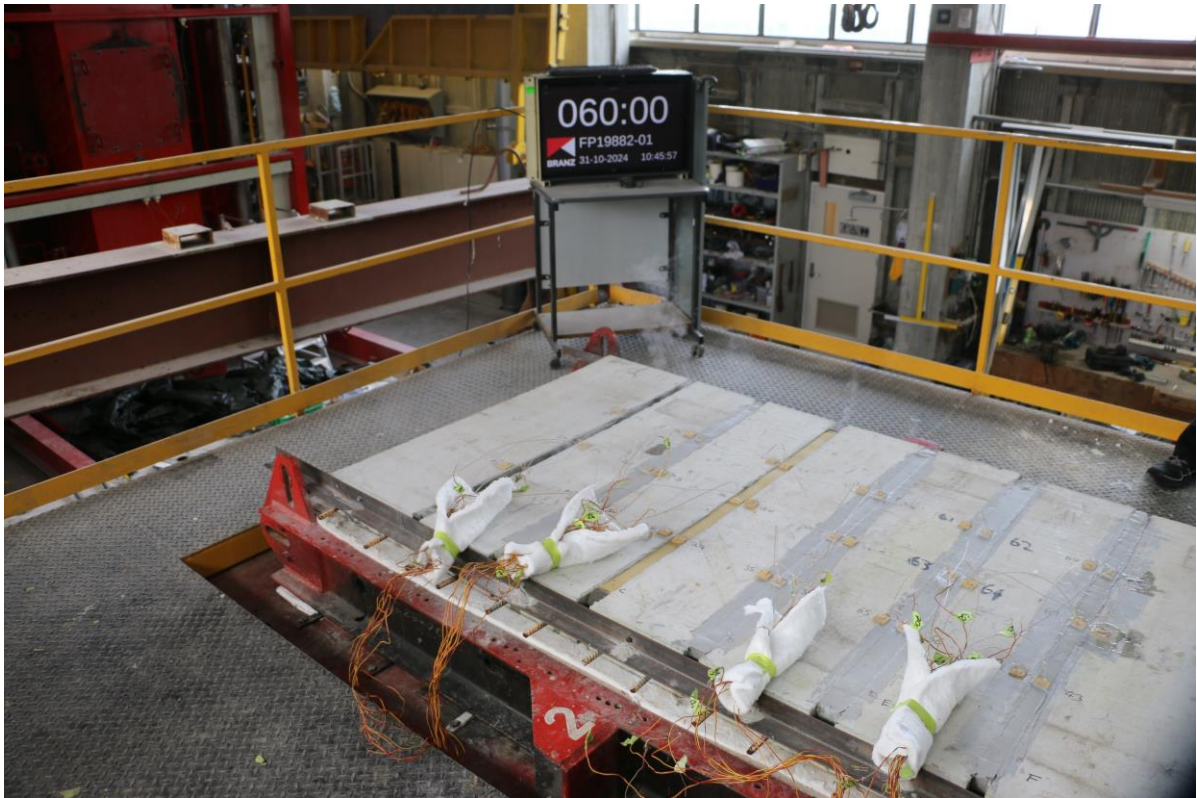
Photo 4: The Unexposed Face of the Test Assembly After a Duration of 120 Minutes
