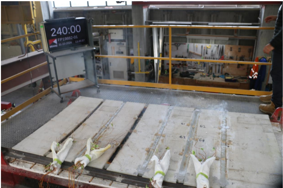
Photo 6: The Unexposed Face of the Test Assembly After a Duration of 240 Minutes
