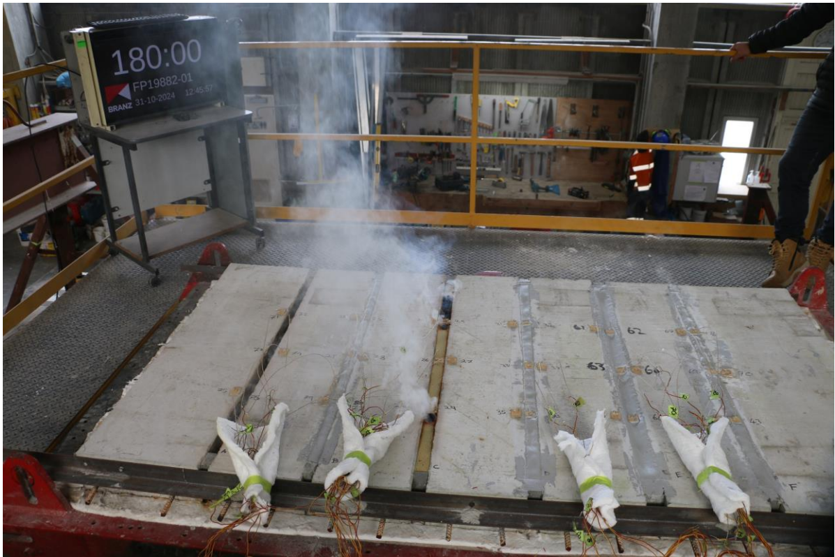
Photo 6: The Unexposed Face of the Test Assembly After a Duration of 240 Minutes
