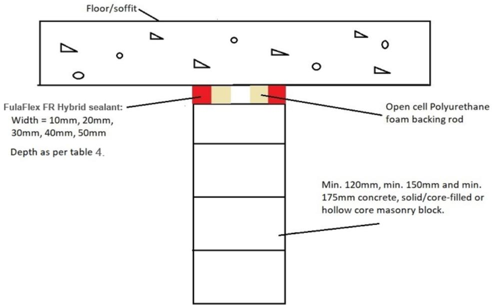
**Figure 4 Head joints in concrete walls with sealant flush on both sides**
