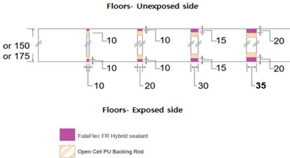
**Figure 2 Control joints with H.B. Fuller FulaFlex FR sealant caulked on both sides in concrete floors**
