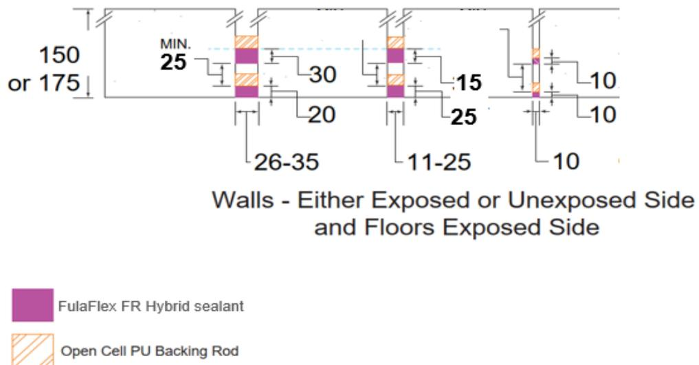
**Figure 3 Double caulked control joints in concrete walls or floors**
