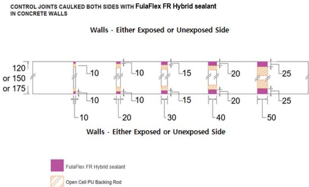
**Figure 1 Control joints with H.B. Fuller FulaFlex FR sealant caulked flush on both sides in concrete walls**
