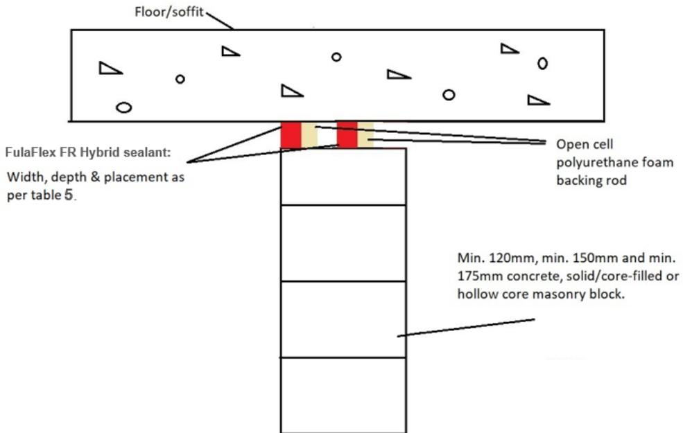
**Figure 5 Double caulked head joints in concrete walls**
