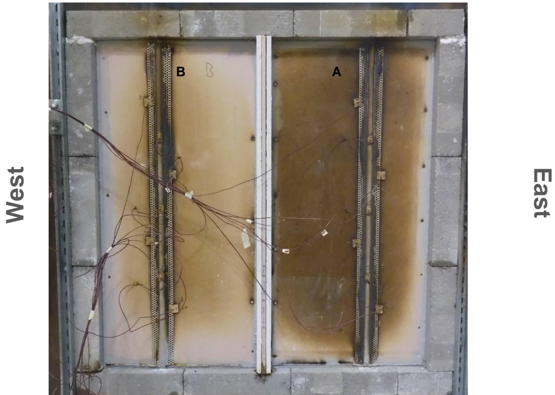
Figure 17 Unexposed face of the specimen at the end of the test
